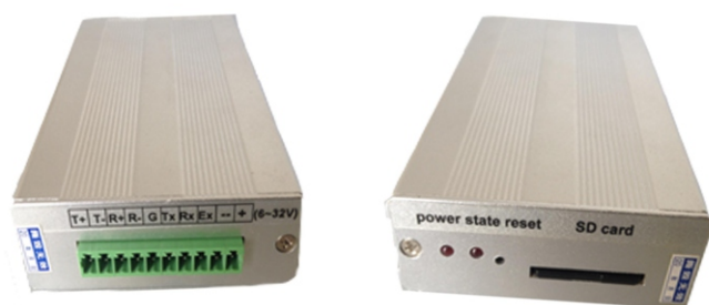
ADR侧面图(102mm × 70mm × 22mm)
